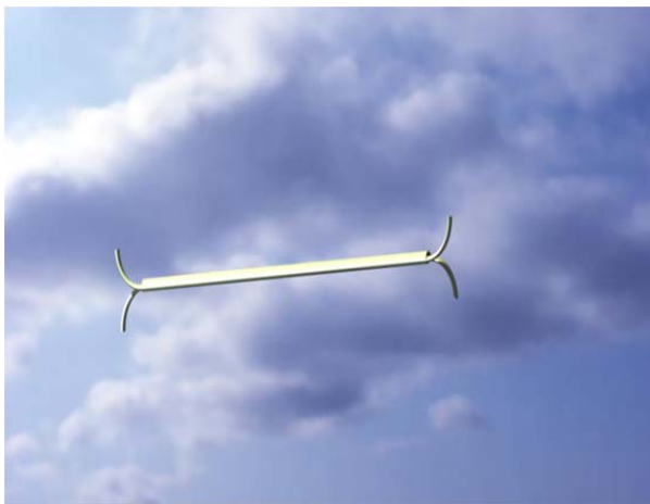
Fig. 2: Split Blended Winglet
